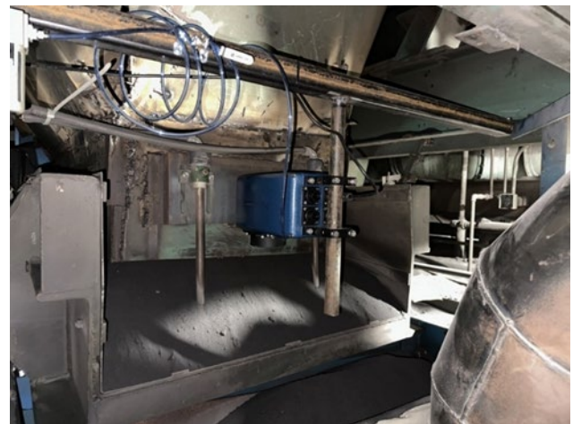
Figure 2. Optical moisture sensor and conductivity probes.
